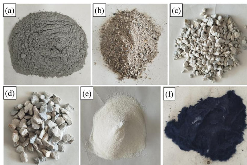
Figure 1. Ingredients of concrete mixture; (a) cement; (b) sand; (c) fine gravel; (d) coarse gravel; (e) superplasticizer; (f) waste fibers
