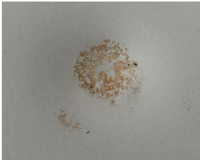
Figure 8. Untreated sample, after the impact test
