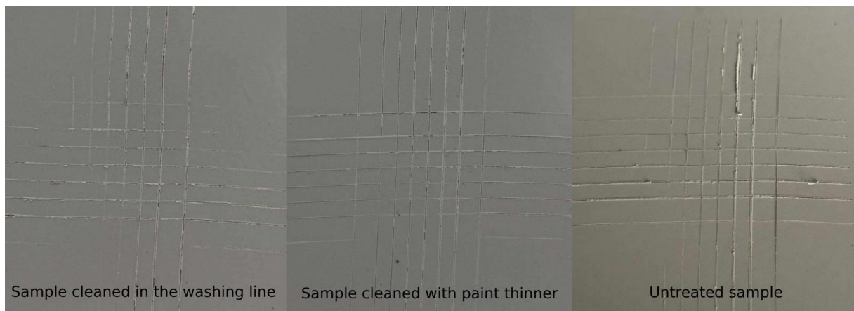
Figure 9. From left to right: Washing line sample, paint thinner sample, and untreated sample cross-cut test results
