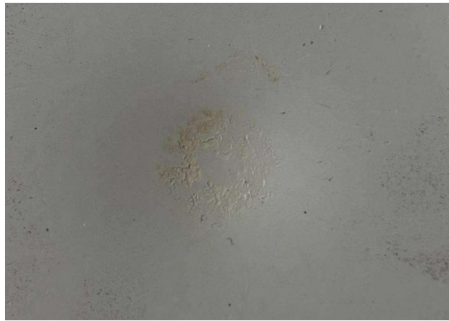
Figure 8. Sample wiped with paint thinner, after the impact test
