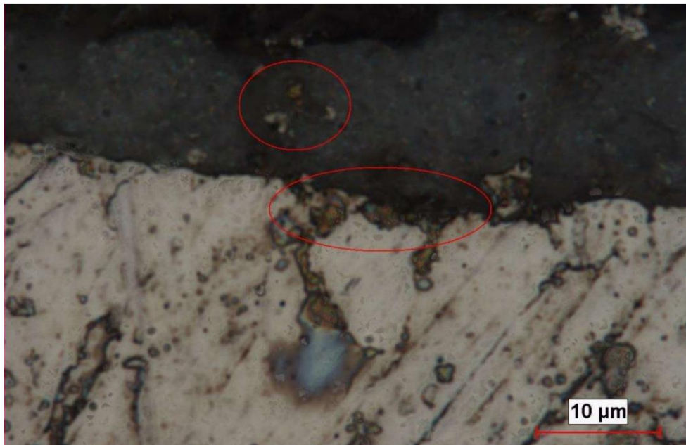
Figure 17. Residual substances between the metal surface and the paint for the untreated sample
