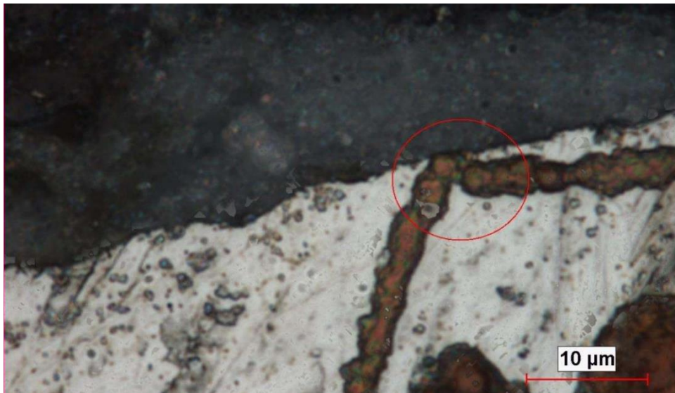
Figure 16. Residual substances between the metal surface and the paint for the untreated sample
