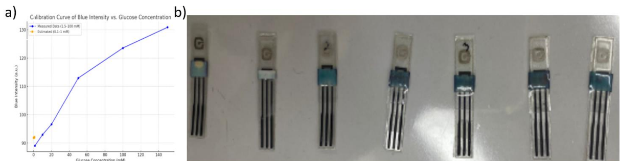
Figure 3. Calibration curve between glucose concentration and blue color intensity (a) Blue color change in glucose colorimetric measurement (b)
